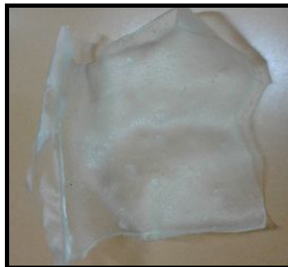
Figure 2: Film of starch made with glycerol and a solution of acetic acid 3% V/V.
