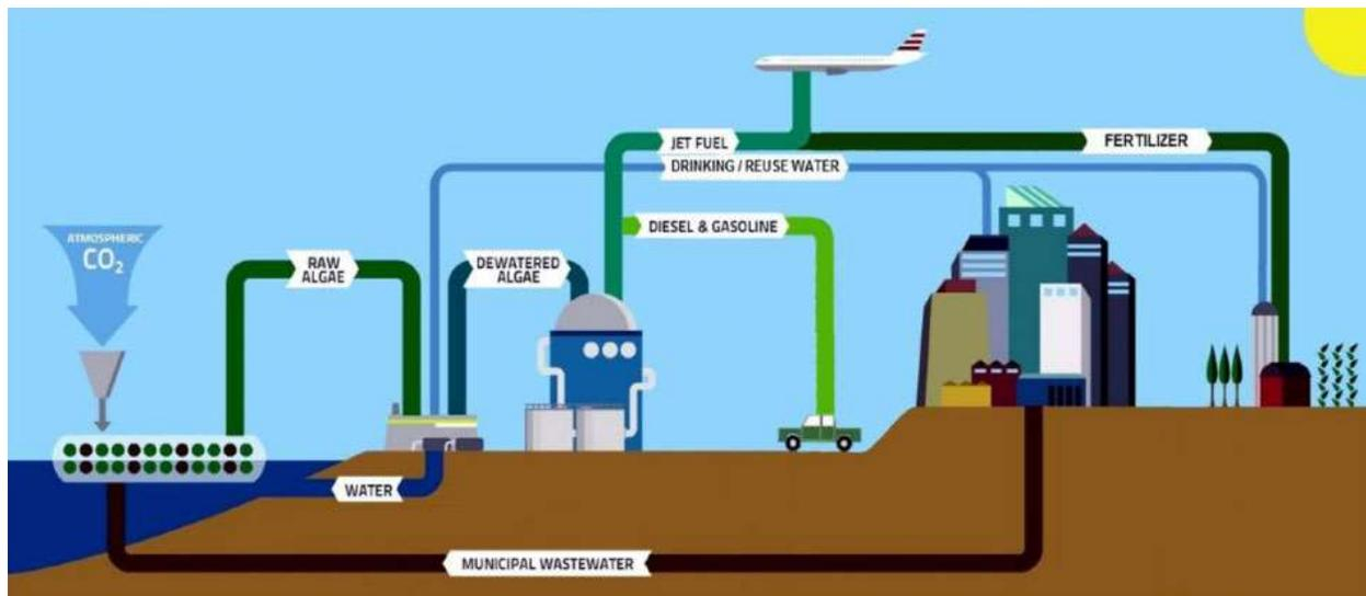
**Figure 3.** Wastewater process treatment using microalgae (18).
