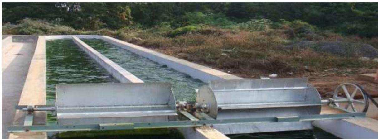
**Figure 2.** Mass cultivation of microalgae using local microalgae strain at CSIR- IMMT Raceway pond (Capacity 30000 L) (15).
